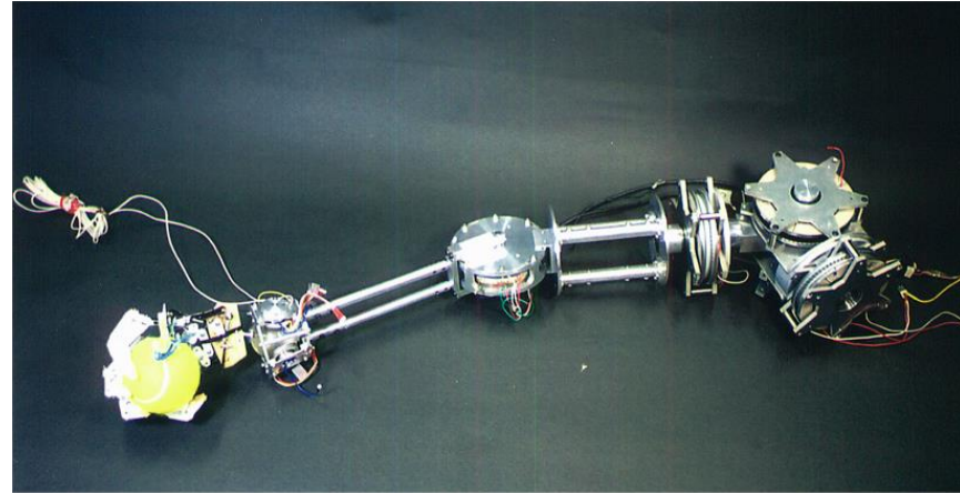
Artificial arm by using spherical ultrasonic motor Tokyo Univ. of Agriculture and Technology (東京農工大学／TUAT)
